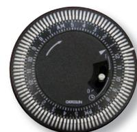
Set the correct time against the arrow. Push the tappets out for any time you want the water tank to heat (several hours during off-peak times). The switch should be left in the middle (timed), rather than 1 (heating constantly) or 0 (off constantly).
